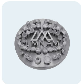
Sample Name: Dentures Sample Material: Titanium Alloy Application: Medical Dentistry
